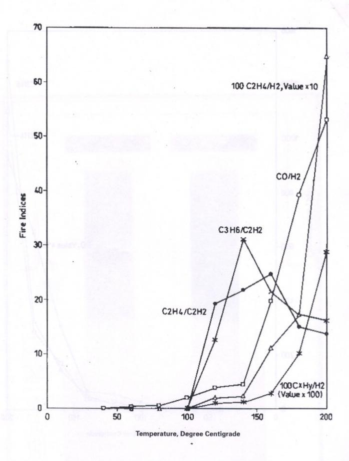
Fig. 5: Variation of fire indices with temperature
