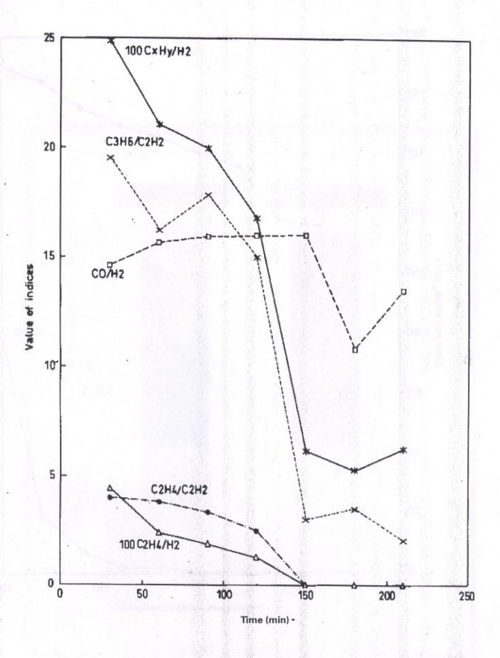
Fig. 3 : Variation of fire indices with time at a constant temperature 150 °C
