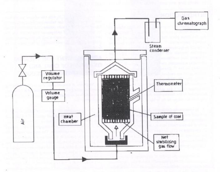
Fig. 1: Diagram of the device for thermal oxidation of coal in air
