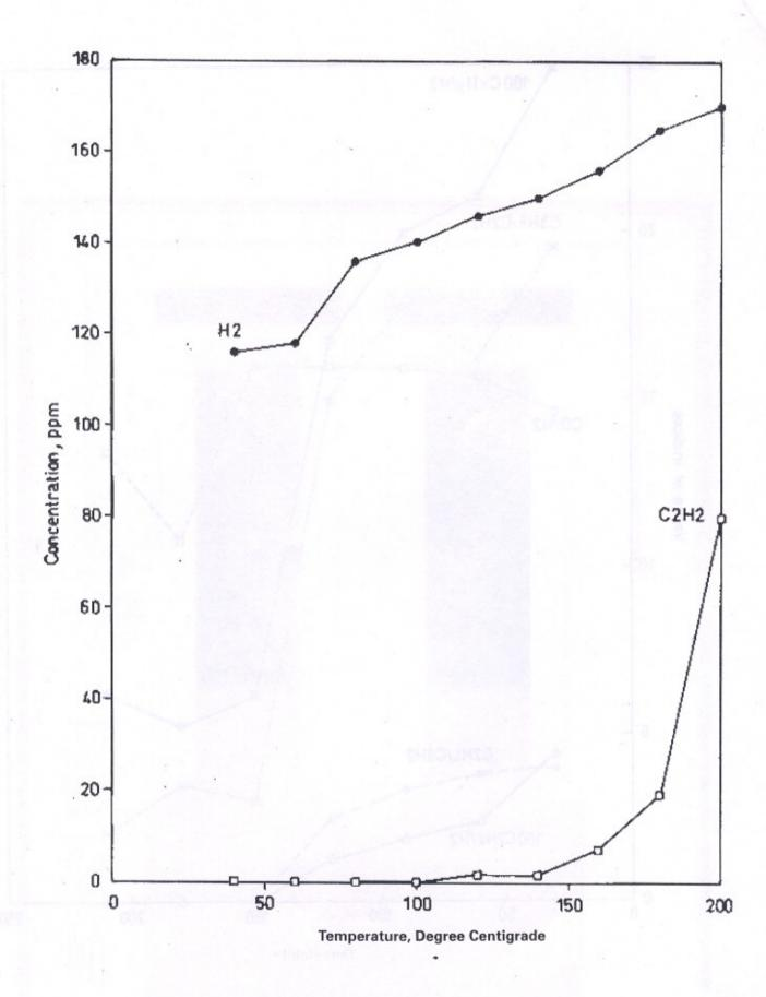
Fig. 4a: Variation of gas concentration with temperature
