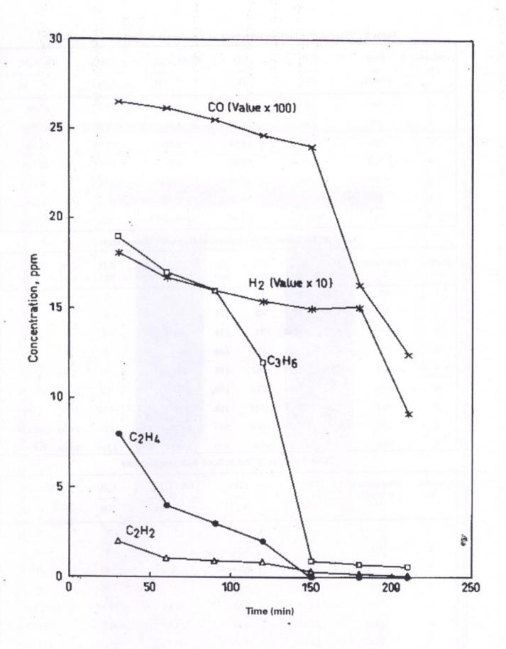
Fig. 2 : Variation of gas concentration with time at a constant temperature 150  $^{\rm o}{\rm C}$
